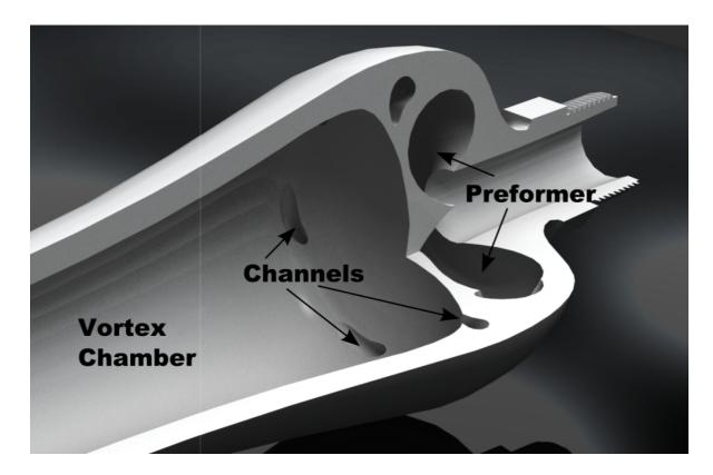
Figure 1 Vortex Chamber of a REALice Wall Unit
