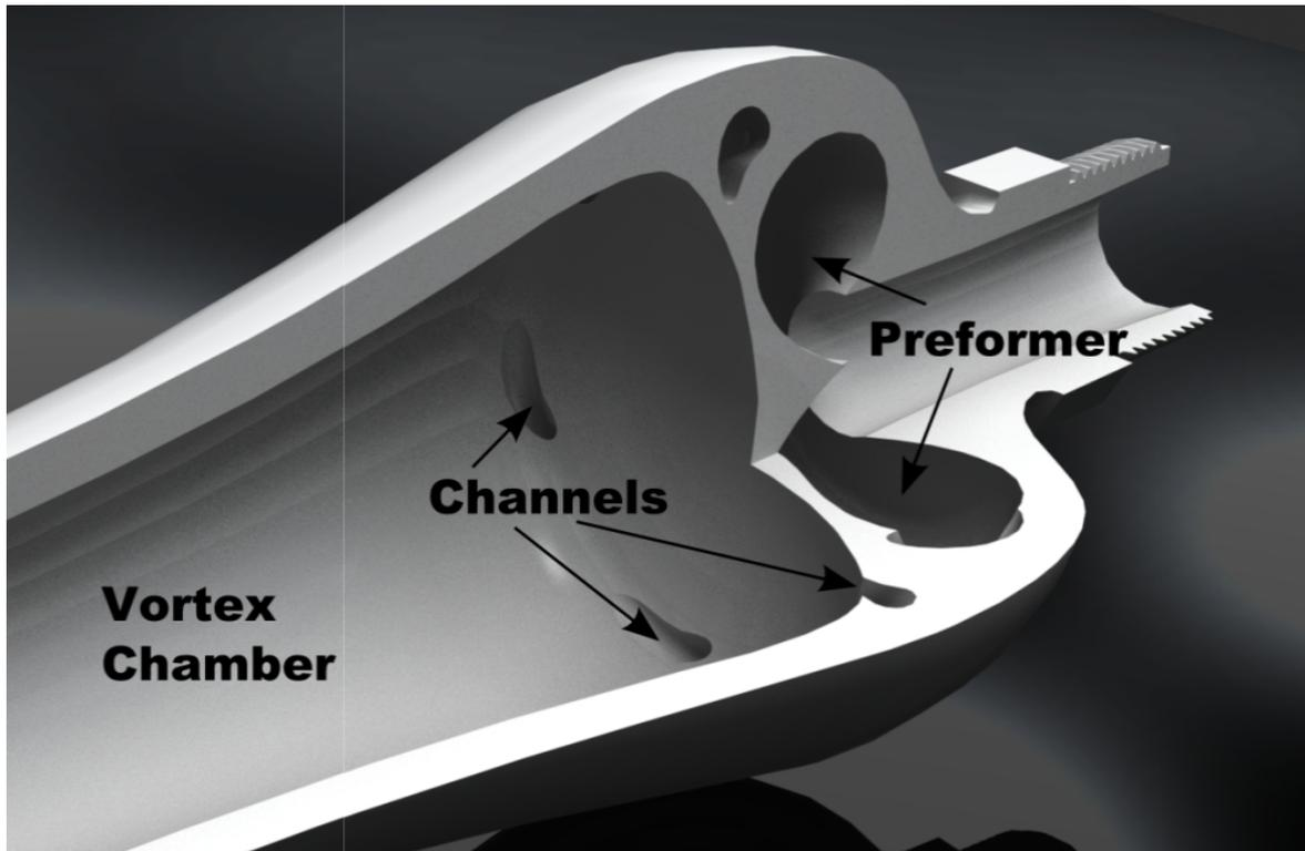
1. **Pre-former.** The inlet of the vortex generator provides a smooth outward direction of the flow through toroidal motion toward a set of well-defined channels.
