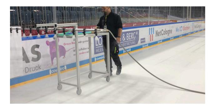
We use a... (paint skid, spray boom or elevated spray boom as pictured above\*) to build our ice – can we continue to use that to make ice? Yes, no problem! Just make sure ALL water is treated through the REALice system. However... we strongly recommend that you build the ice using the REALice handheld as you will build the ice in thin, dense layers – and you will be surprised at how quickly you are able to build your surface up.
